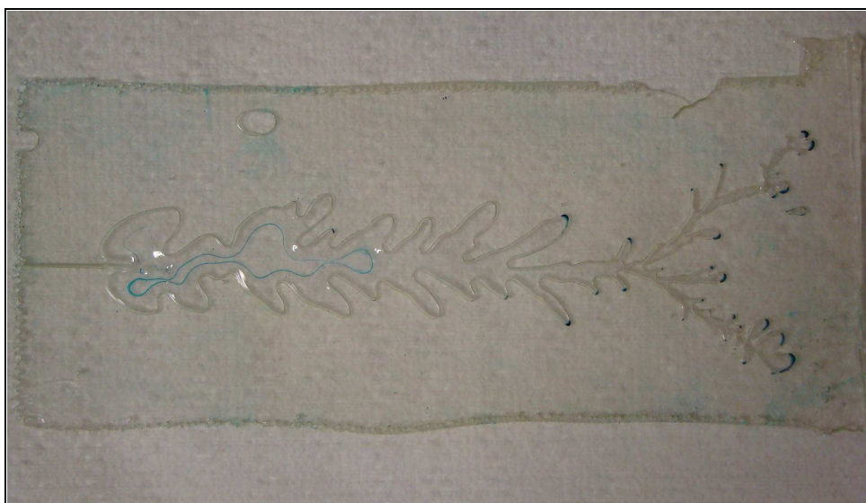
Figure 13: Cured Ebecryl-230 Branching Structure
