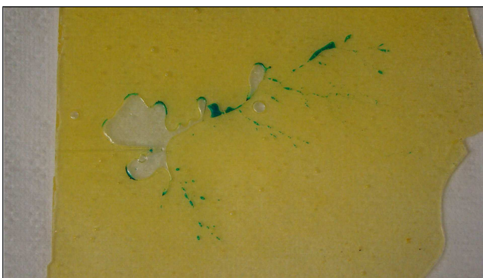
Figure 15: Cured CN-151/Styrene Branching Structure
