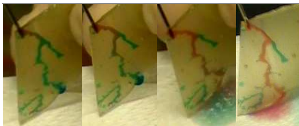
Figure 30: Fill and Flow Sequence Through Small Length Scales
