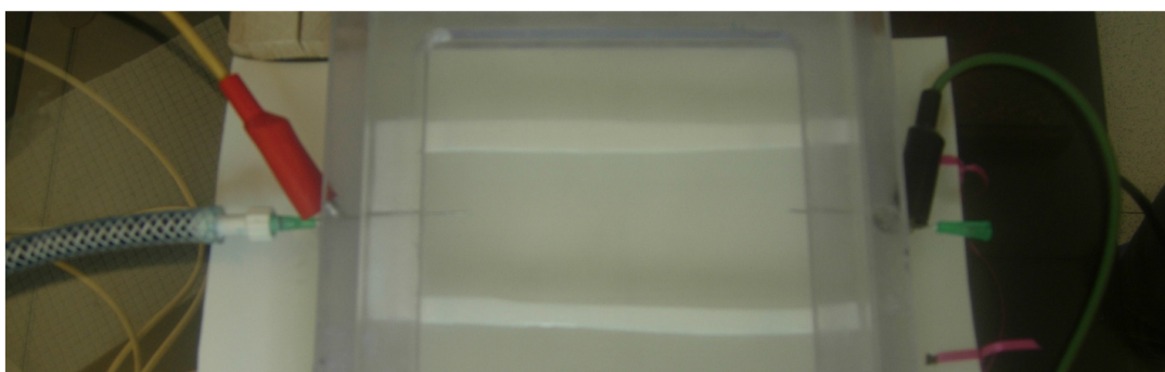
Figure 23: Close-up of UV-Cure Hele-Shaw Cell
