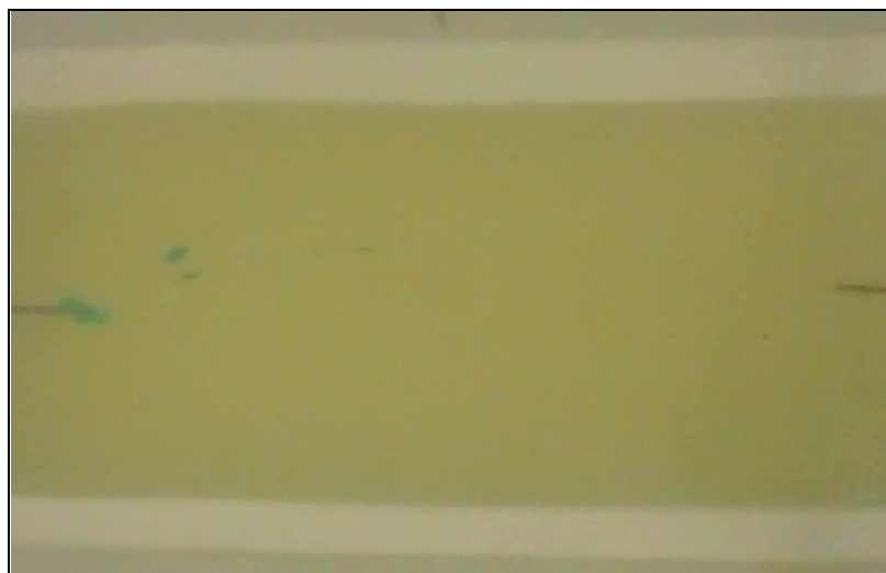
Figure 25: Premature Cure Example
