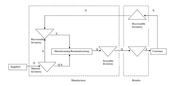
Figure C.1: The Recovery and Remanufacturing Process
