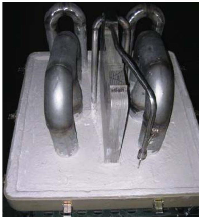
Figure 37. Photographs of the auxiliary power unit box that was constructed to house the two plasma reformers (top). An image of the internal M-shaped reactor enclosures (bottom).
