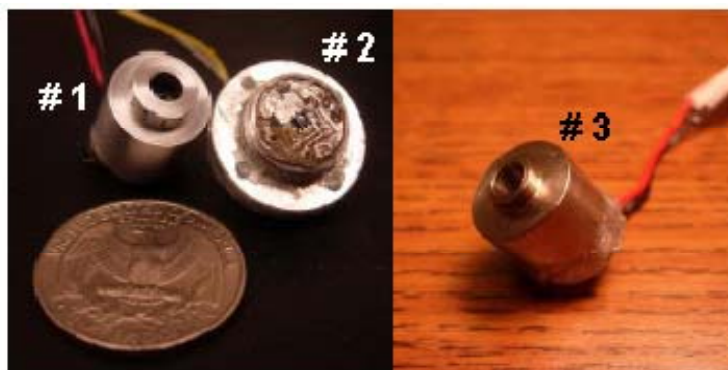
Figure 5.5 The casing material of ICP devices. The casing material of the implant #1(Type SD_Cap_C), #2 (Type ED_Cap_C), and #3 (Type SD_Cap_C) was stainless-steel, aluminum, and titanium, respectively.
