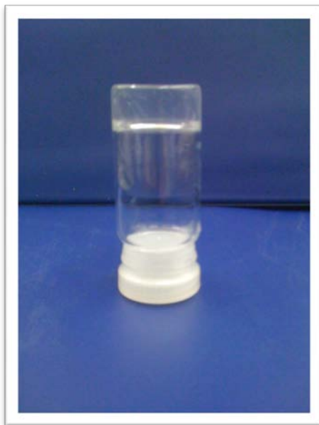
Figure 53: Self-supporting AK-16 hydrogel, prepared by adding NaCl to a 5 mg/mL solution of AK-16 to yield a 2 M NaCl AK-16 hydrogel.
