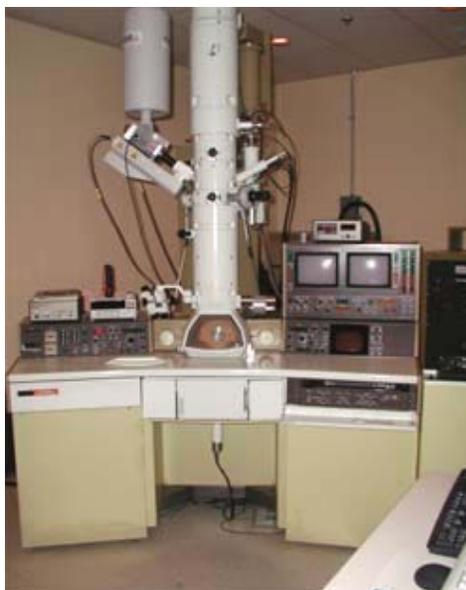
Figure 3.15: An image of a JEOL 2000-fx TEM [187].
