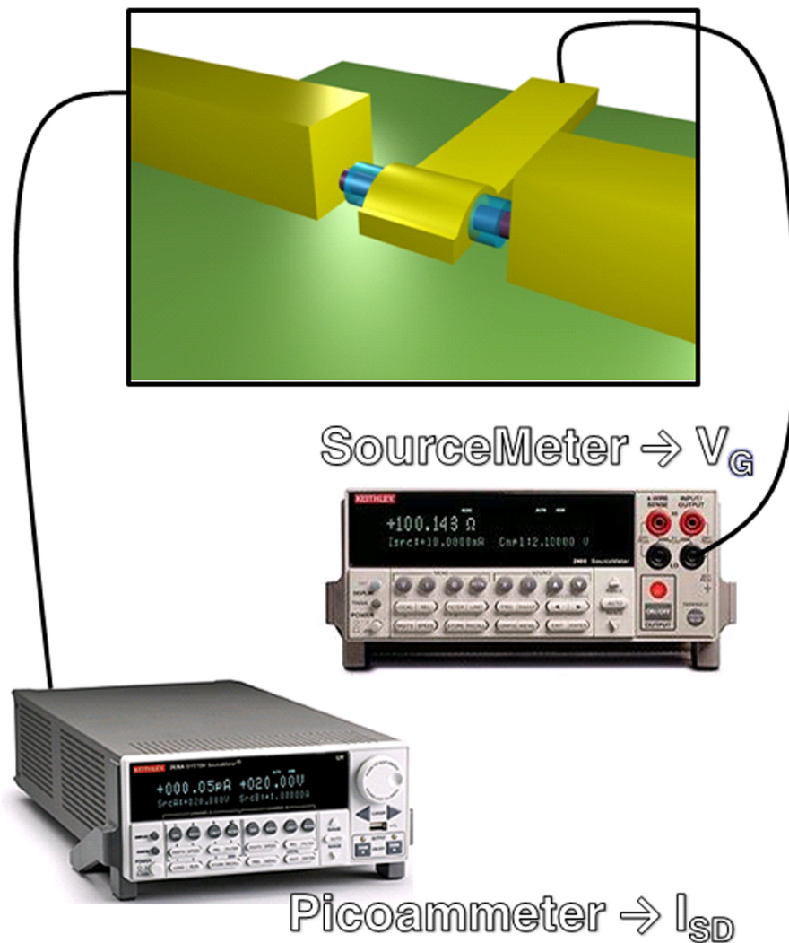
FIGURE 6.4: Illustration of the experimental setup used for gated measurements of I-V through the nanowire core. A sourcemeter is attached to the gate while a picoammeter is attached to the source-drain of the nanowire channel. A gate voltage ( V_G ) is applied directly to the wrap gate electrode, then removed to collect current, as shown in Figure 6.6
