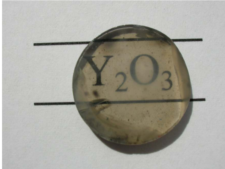
Fig. 3-1: Picture of the transparent yttria sample used in the experiments.
