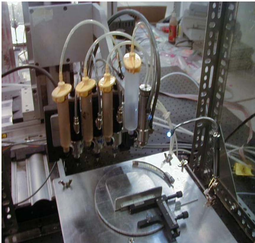
Figure 1-6: Direct cell writing system with multinozzle capability
