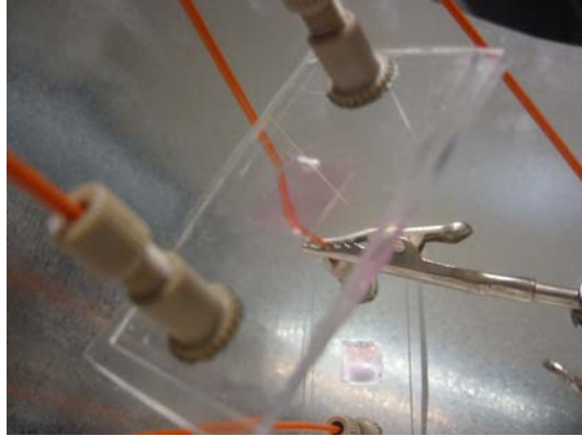
Figure 6-14: A fully perfused tissue chamber with drug/media
