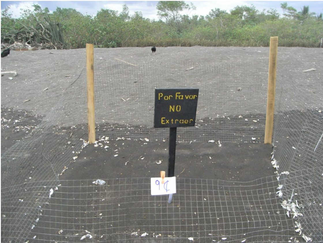
Figure 2.5. Example of a “Closed Plot” ( 2x2 m) in the low beach zone, below the high tide line of Ostional Northwest Costa Rica.
