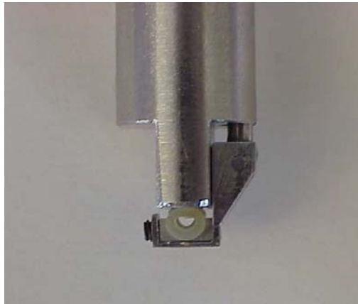
Figure 5.7. Hand-held tonometer tip. Silicone tubing is placed in the U-shaped support structure
