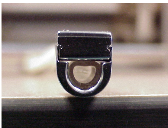
Figure 5.11 Front view. Miniature tonometer for chronic implantation.
