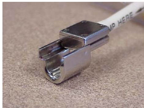
Figure 5.10. Disassembled tonometer shows the idea of artery fixation between U-shaped and flat structures.
