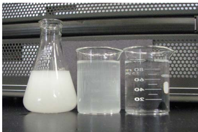
Figure 6-17: From left to right: 1 mg/mL silica suspension, 0.1 mg/mL silica suspension and pure tap water
