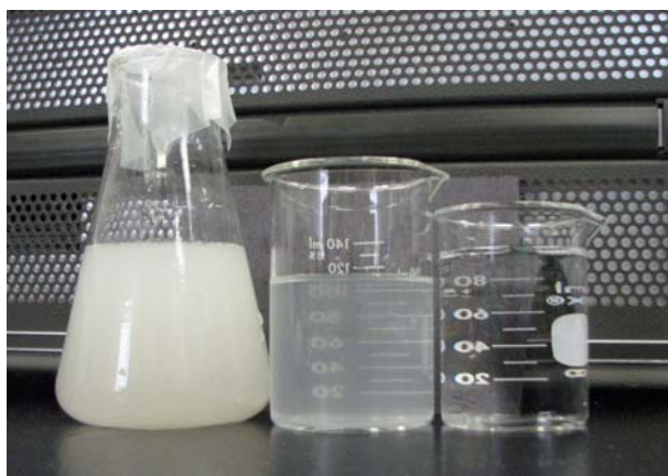
Figure 6-20: From left to right: 1 mg/mL clay suspension, 0.1 mg/mL clay suspension and pure tap water
