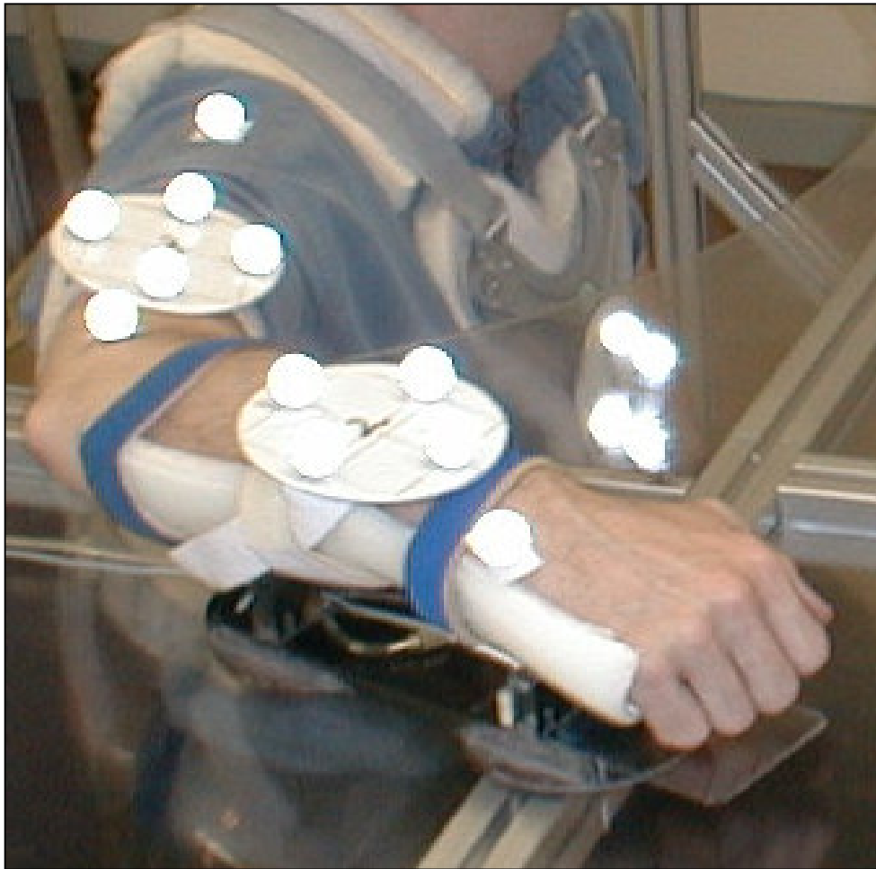
Figure 7: Illustration of marker placement, air bearing carriage, and chest harness. Note that the marker bodies on the upper and forearm were not needed because these segments did not rotate.
