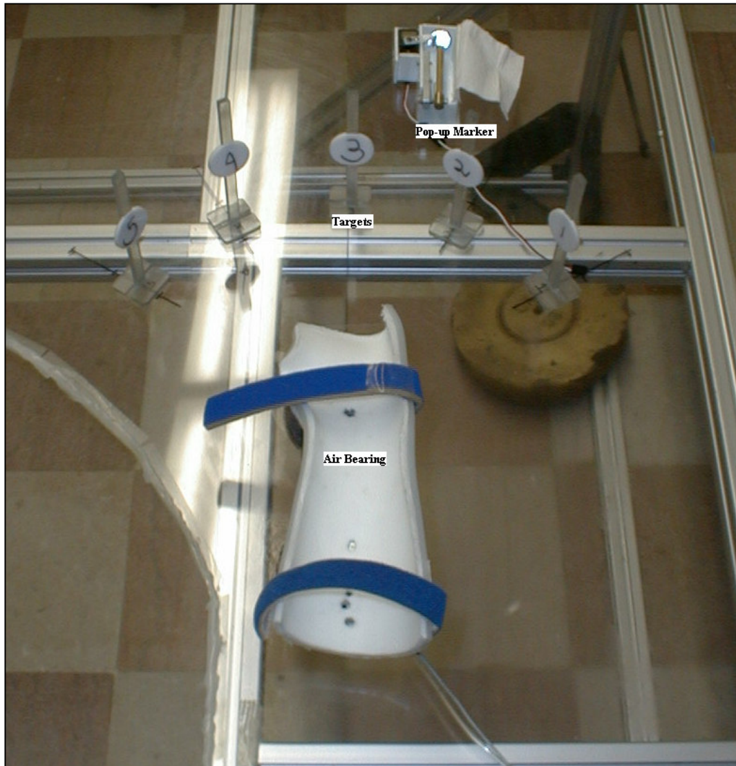
Figure 8: Targets are located at angles of 30°, 60°, 90°, 120°, and 150° degrees relative to the wrist start position. The subject sat in their own wheelchair; the table height was adjusted until the upper arm is abducted 90° degrees in the frontal and transverse planes. The forearm was flexed 90° degrees and strapped into the air bearing carriage. Subjects were asked to acquire each target five times consecutively from wrist start position. The 30°, 60°, 90°, and 120° degree target were acquired fives time from while the subject started while pointing at the 150° degree target.
