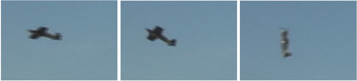
Figure 5.11: The transition from cruise flight (left), through the stall regime (center), and into hover mode (right) is achieved autonomously.
