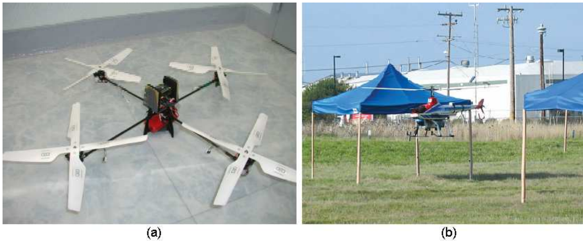
Figure 2.5: (a) ANU's X4-Flyer is a quadrotor platform using differential thrust for attitude adjustment. Reprinted from [23]. (b) UC Berkeley's RMAX UAV is used as a testbed for implementing collision avoidance and navigation algorithms in urban environments. Reprinted from [50].
