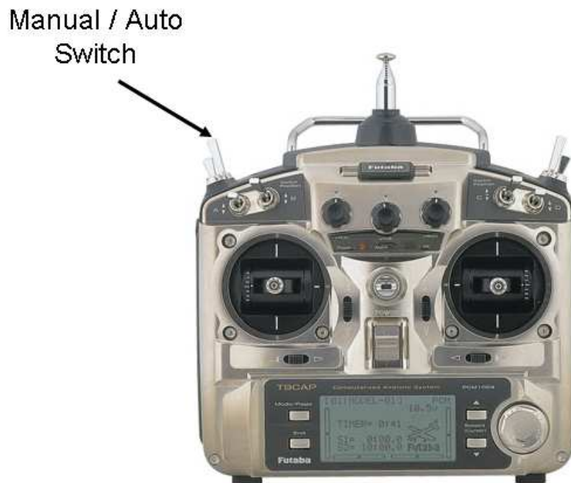
Figure 5.4: A switch on the remote-controlled transmitter was used to toggle back and forth between manual and autonomous control.
