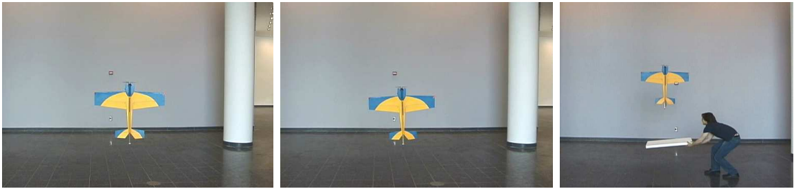
Figure 5.17: The first two images in the above sequence show the hybrid MAV in a fully autonomous hover at a height of 36 inches at 6 seconds apart. In the third image, a board was placed under the MAV's tail which caused the controller to adjust the MAV's height to 36 inches above the board. This was used to show that a constant throttle setting was not used to perform altitude hold.
