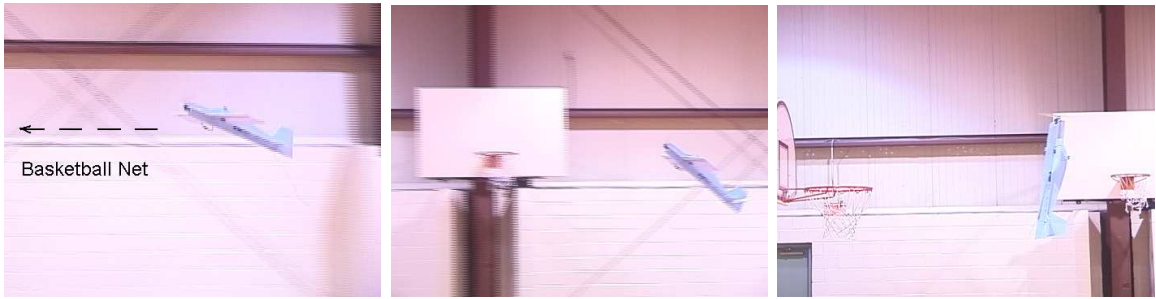
Figure 3.7: Our MAV prototype with a 1 meter wingspan manually transitions from cruise flight (top left) through the stall regime (top middle) and into a hovering position (top right) to avoid a collision with a basketball net.
