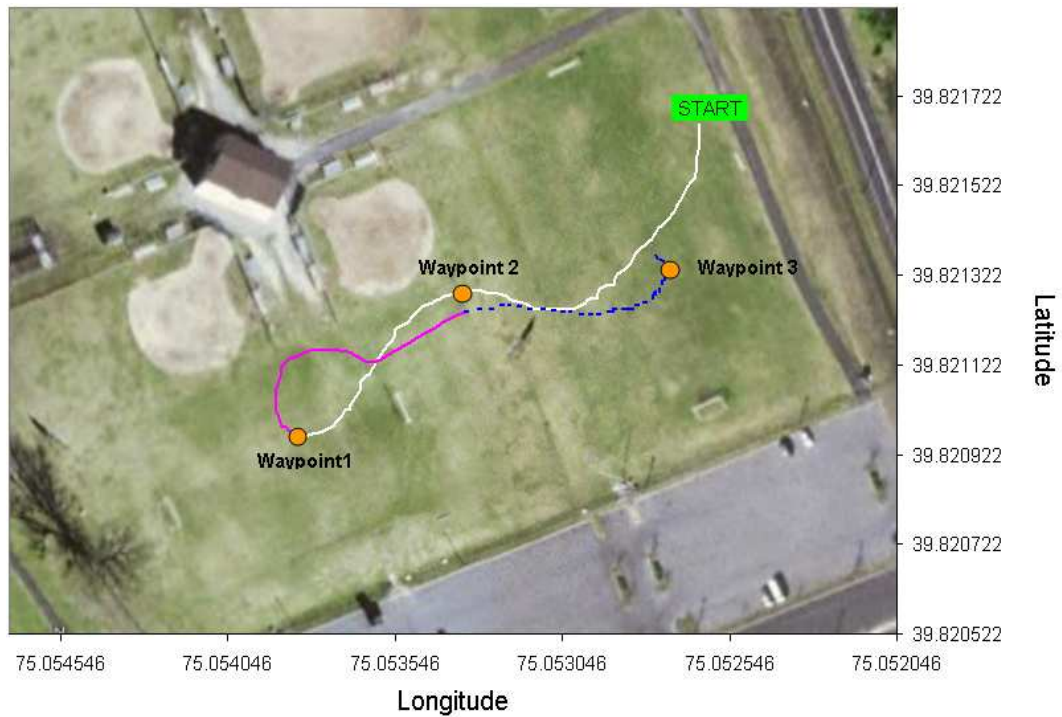
Figure A.2: A Garmin GPS 18 5Hz receiver is interfaced with the FCS to perform autonomous waypoint navigation.
