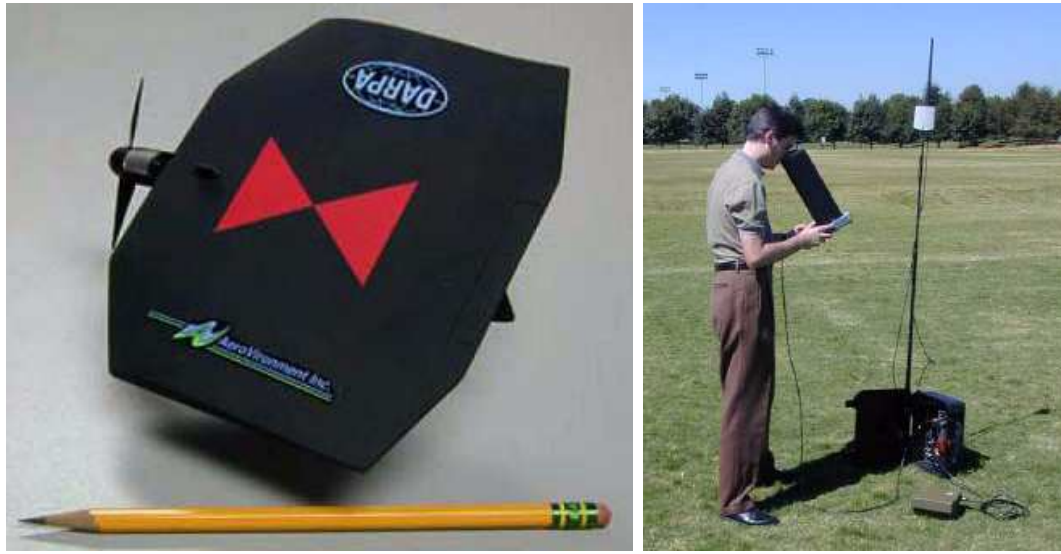
Figure 2.1: AeroVironment, Inc.'s Black Widow is flown under human-control from a remote location. The human pilots the MAV by looking at raw video transmitted from the wireless camera onboard the MAV. Reprinted from [16].
