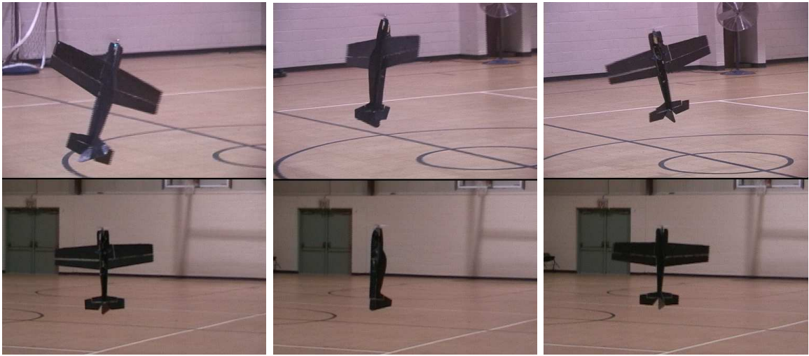
Figure 5.9: A skilled human pilot hovers a fixed-wing aircraft in a small gymnasium and struggles to maintain a vertical orientation (top). Under autonomous control, the same aircraft is able to sustain a hover while remaining fixed in the vertical position (bottom).
