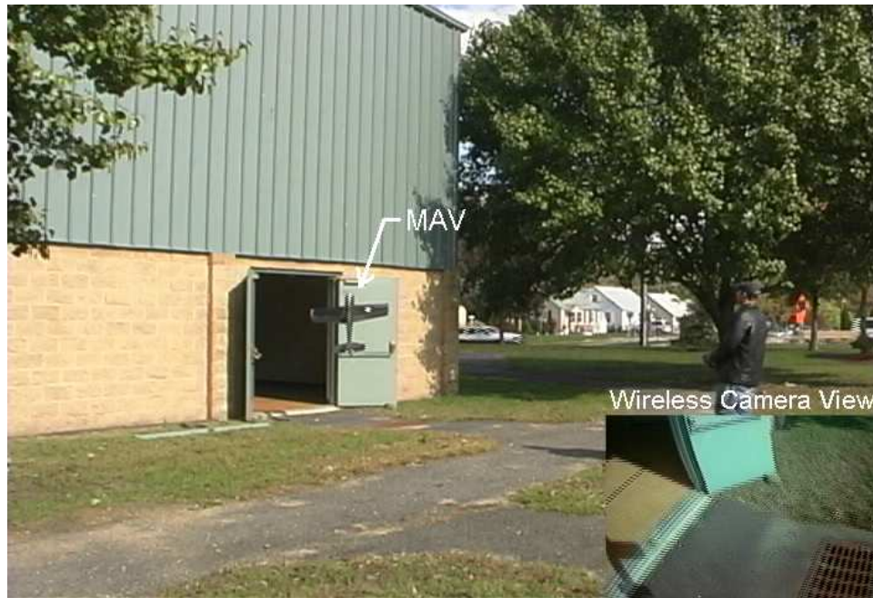
Figure 6.1: A fixed-wing MAV transitions to hovering mode to gently maneuver itself through a small opening of an urban structure. Inset: once inside, the onboard wireless camera is used to capture and transmit surveillance images.
