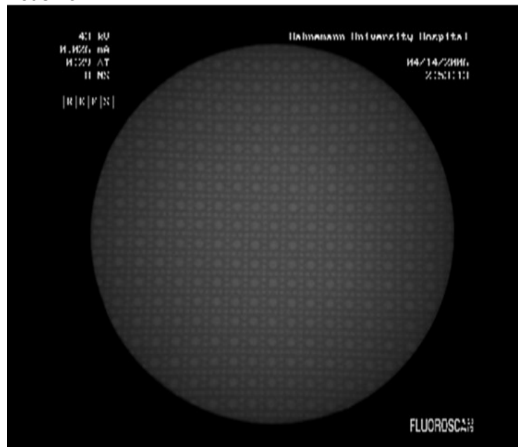
Figure 7.3: The grid images used during C-arm calibration a) the radial errors from the center of the imaged were used to perform the pincushion correction b) image after pincushion correction
