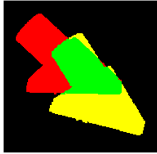
Figure 6.9: The red and green area shows the object silhouette transformed by the ground truth. The yellow and green area shows the object silhouette transformed by the computed transformation. The minimum normalized overlap \Gamma = 0.462 .
