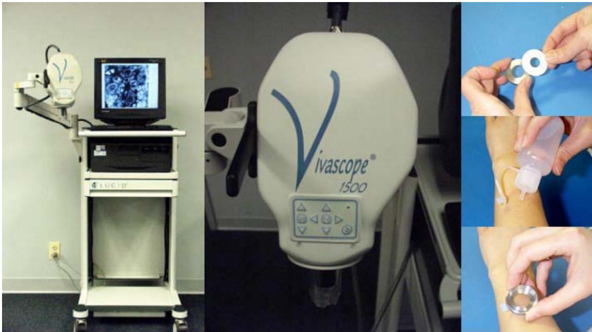
Figure 8 – Image of the commercially available scanning laser confocal microscope the Lucid Vivascope 1500. Current standard wavelength is 830nm and experimental wavelengths used were 785nm and 405nm for their ability to do both reflectance mode imaging in addition to fluorescence mode imaging. Note, these are fluid immersion objectives and both oil and water objectives were used to see if there was a significant difference in resolution between the microscopes. NOTE example of tissue ring and coverslip mechanism that attaches microscope to human skin is a part of the optical design and optical path of the microscope (Images courtesy of Lucid Inc.).
