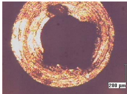
Figure 4.3: EDM positioning problem
