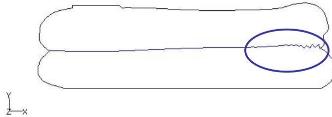
Figure 3.37: Effects on the position of the interface when high flow is applied
