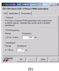
Figure 5.4 The PWM inverter control circuit (a) and PWM control module (b) in MATLAB Simulink for the dSPACE DS1104 DSP card
