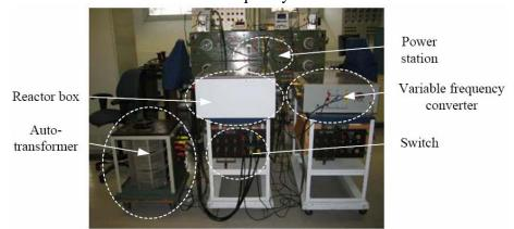
Figure F.7 The hardware setup of the three-phase ac/dc system with a three-phase variable frequency converter
