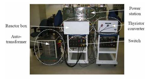
Figure E.3 The hardware setup of the three-phase ac/dc system with a three-phase thyristor converter
