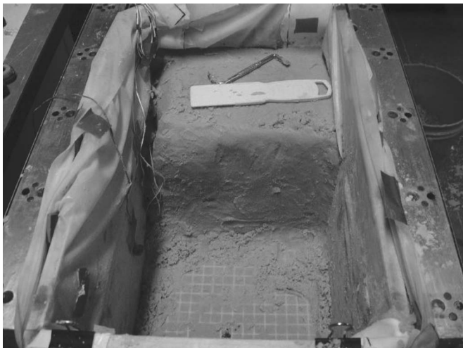
Fig. 7. Photograph of model excavation and uniformly grouted soil
