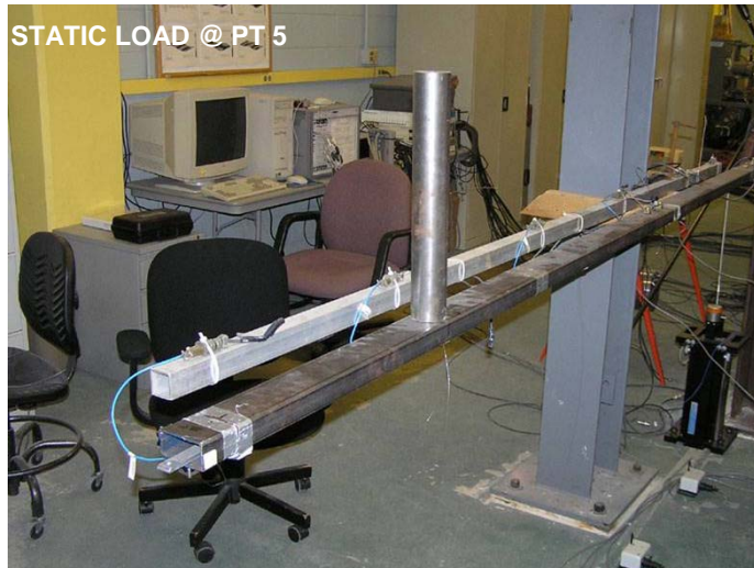
Figure 4-23 Static test on the cantilever beam
