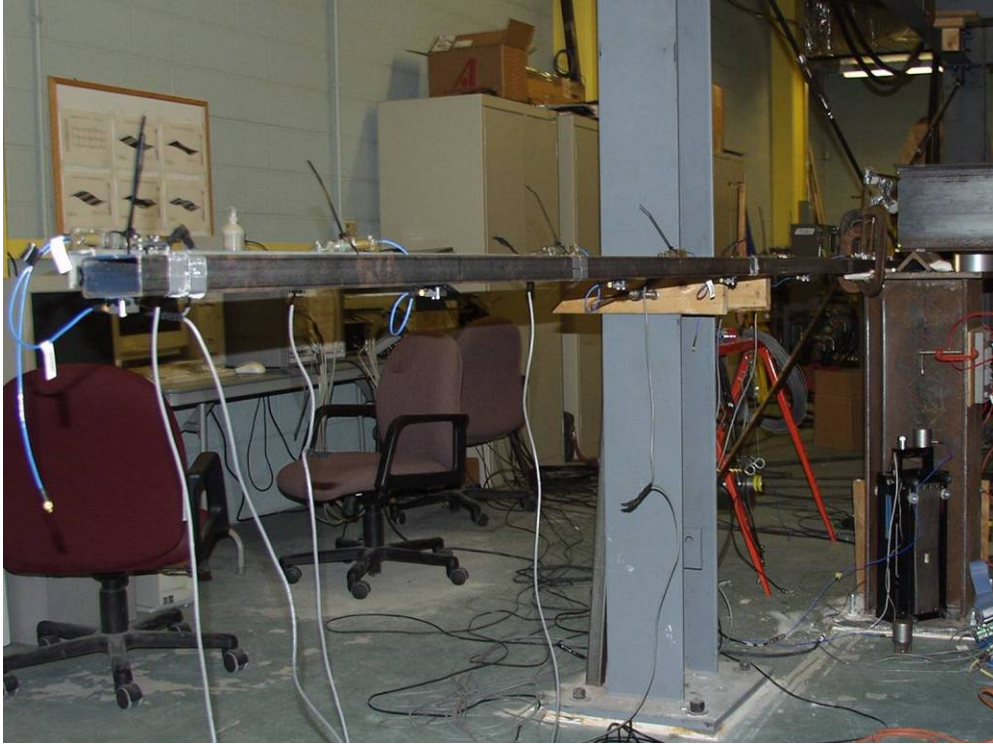
Figure 4-8 Test beam setup 1 with fixed support
