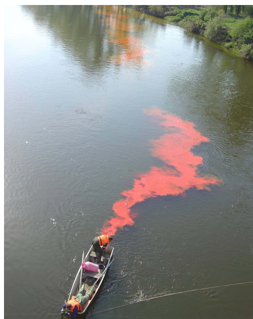
Figure 5 Input of the tracer Red Dye near Němčice, Czech Republic
