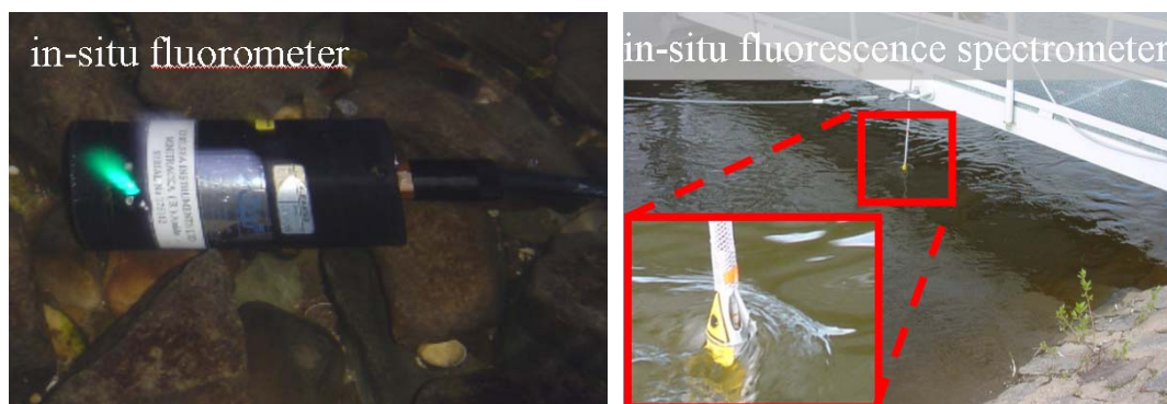
Figure 6 In-Situ measurements of dye concentration.
