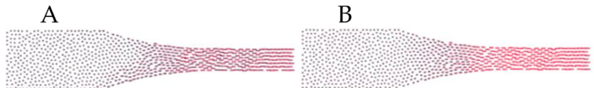
Figure 3.11 (A) Actual particle coordinates and velocities from simulation compared to (B) assumed velocity field for \chi = 0.2 (400 particles)
