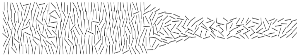
Figure 3.18 Orientation field for a system of ellipse particles during roll compaction
