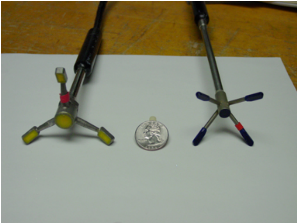
Figure 2 MicroADV (left) and Vectrino (right) head comparison. A quarter is provided for scale.
