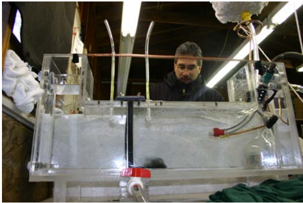
Figure 3. Showing Sloughing After Discontinued Influent Stream
