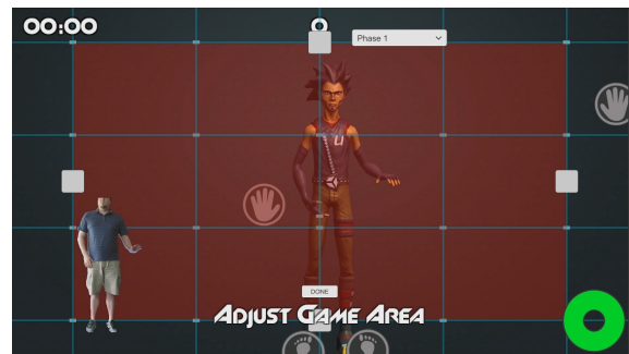
Figure 5.6: A patient with asymmetric arm movement capability will leverage independent extents. Note the mirrored right arm's limited horizontal extension moves the corresponding hand marker all the way to the edge of the screen.
