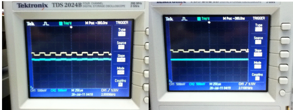
Figure 2.8: Tuning the feedback circuit. In yellow is the signal fed into the feedback circuit: a square wave superimposed on the +15V DC signal. In blue is the output from the feedback circuit. Curves have been offset for clarity. At left, the variable resistor R_1 is set to too high a value, leading insufficient current to flow through the feedback circuit to completely cancel the high-frequency signal. At right, R_1 is set properly. Further zooming in time and in voltage reveals a similarly flat response, even at the near-discontinuous step edges of the square wave input signal.
