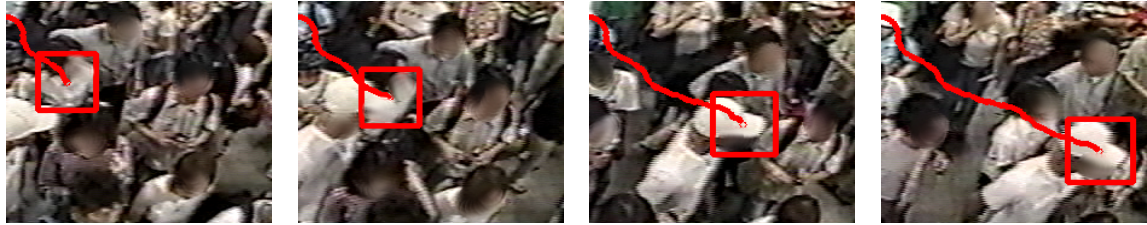
Figure 4.6: Example of a tracking failure due to occlusion.
