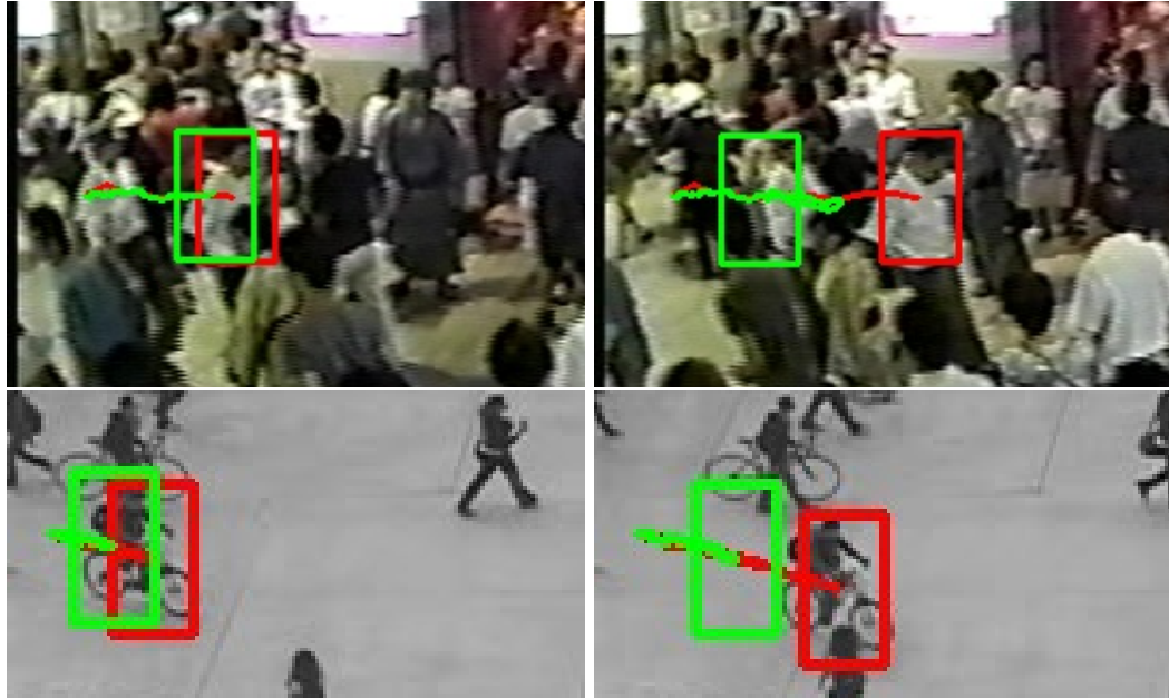
Figure 5.11: Tracking results of anomalous pedestrians from the concourse (top) and UCSD dataset (bottom) using conformance (red) and a crowd model (green).
