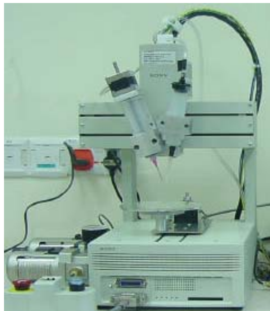
Figure 2.8: RPBOD printing machine set-ups via dual dispensing (Geng, et al., 2003)
