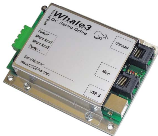
Figure 3.6: Whale3 DC servo drive with integrated connection interface
