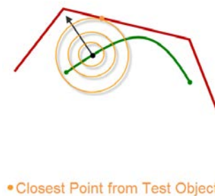
Figure 6 - Explanation of maximum deviation used in 3D deviation analysis in Geomagic Control™
