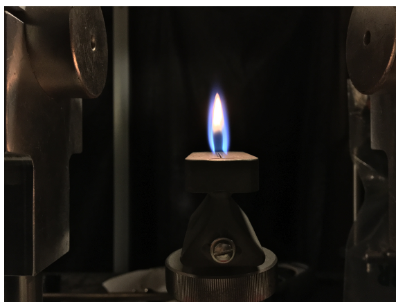
Figure 6.3: Longitudinal path in pre-mixed propane-air slot burner flame.
