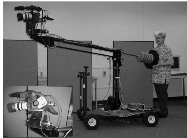
Fig. 2. Operator can boom the arm horizontally and vertically to position the camera. The pan-tilt head ( lower left inset ) provides additional DOFs.
