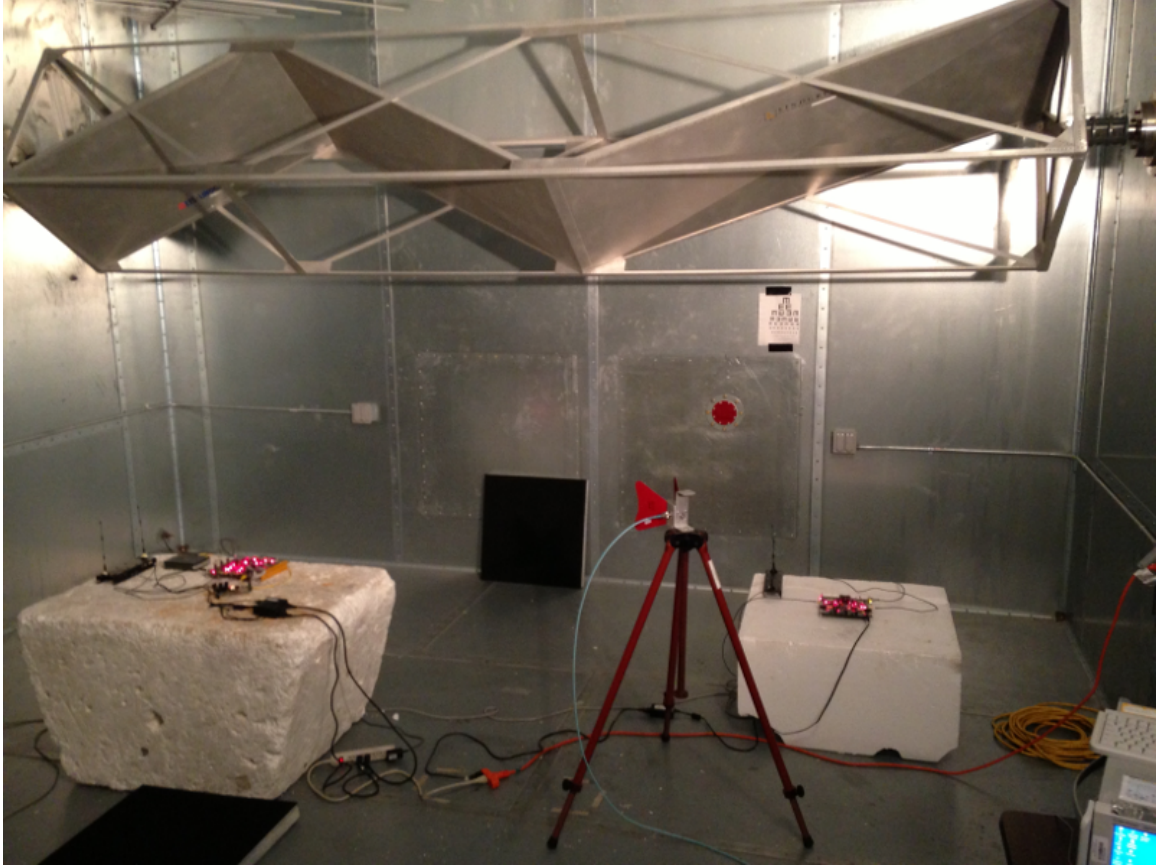
Figure 2.2: Main chamber of the coupled reverberation chambers of the NSWCD. This picture was taken from the doorway connecting the main chamber to the ante chamber. The horizontal Z-fold mechanical tuner along the north wall is shown at the top of the image. One of the horn antennas used for the impulse measurements is on the tripod in the middle of the image. Two of the wireless nodes (described in Chapter 3) are shown on non-absorbing Styrofoam blocks.
