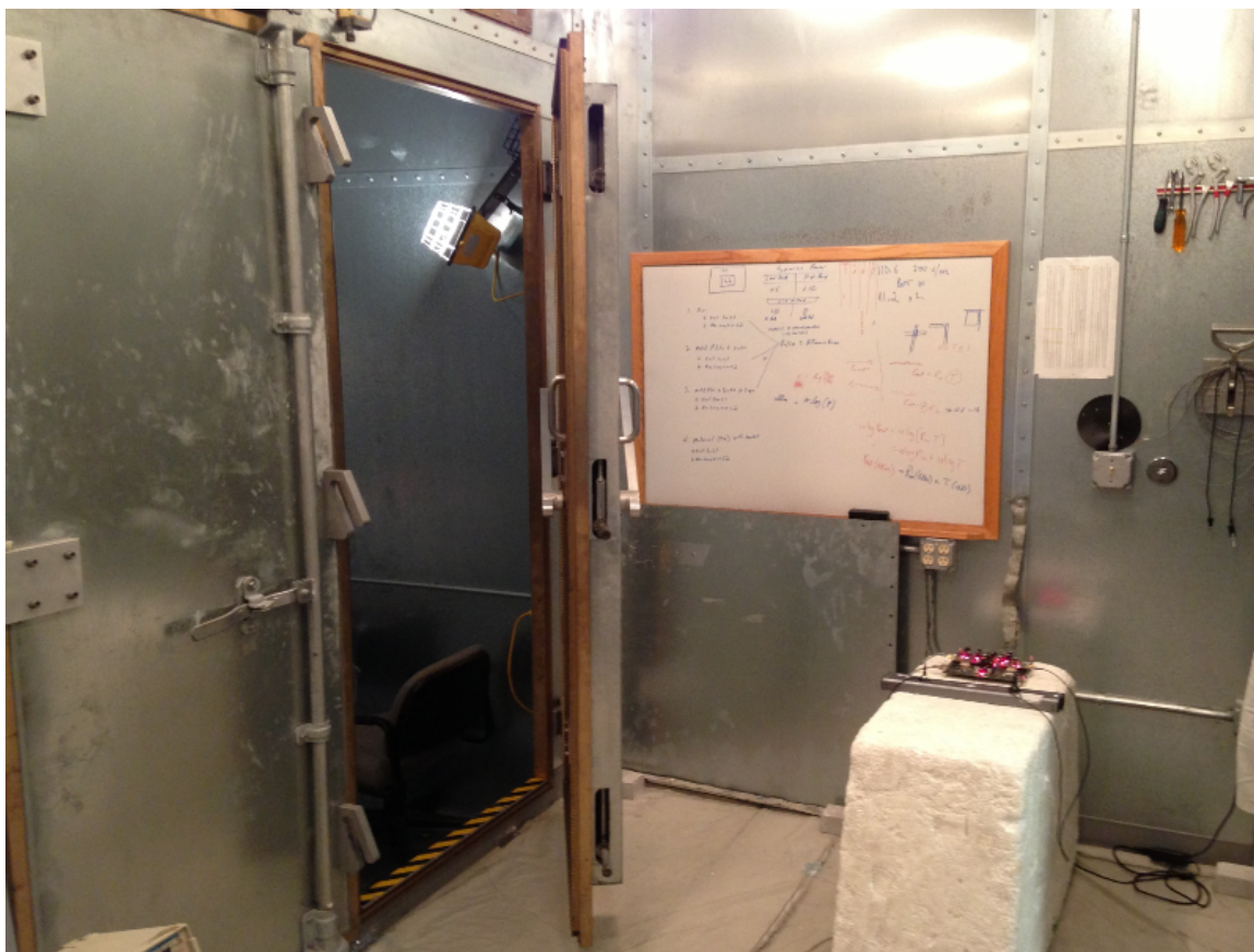
Figure 2.3: Ante chamber of the coupled reverberation chambers of the NSWCCD. This picture was taken from the south east corner of the ante chamber. One of the wireless nodes is shown on a non-absorbing Styrofoam block. The shielded door separating the main chamber and ante chamber is also shown.
