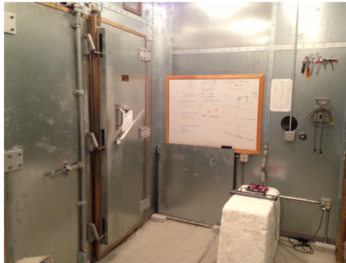
Figure 4.12: Position of the shielded door between the main chamber and the ante chamber for Low Coupling configuration.
