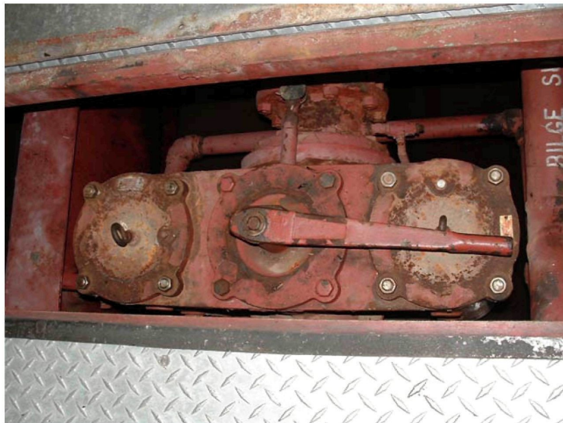
Figure 2. Typical Main Engine Duplex Strainer (Top View)
