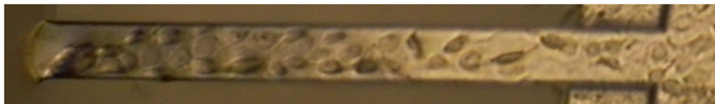
Figure 6-3. Microscope images of the cells cultured on a microcantilever before and after exposure to 8.0-mM M \beta CD. The cells exhibit a flat morphology before exposure (A) and a more rounded morphology after exposure (B).
