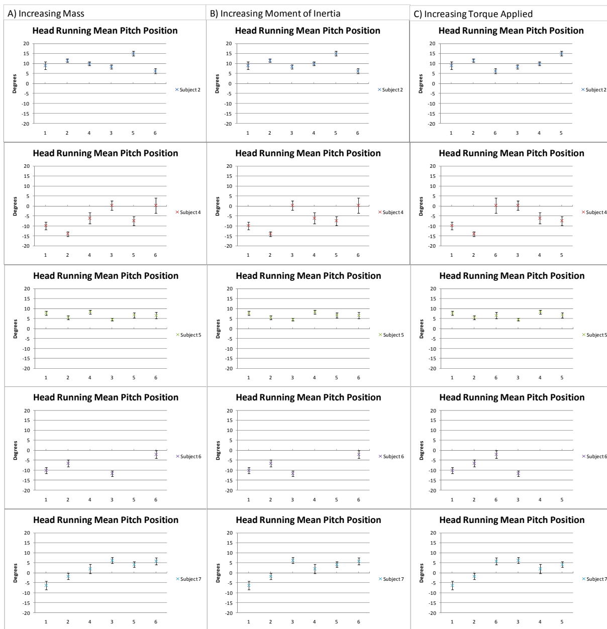
Figure 38: Mean Running Head Pitch Rotation with Standard Deviation for A) Increasing Mass, B) Increasing Moment of Inertia, and C) Increasing Torque Applied
