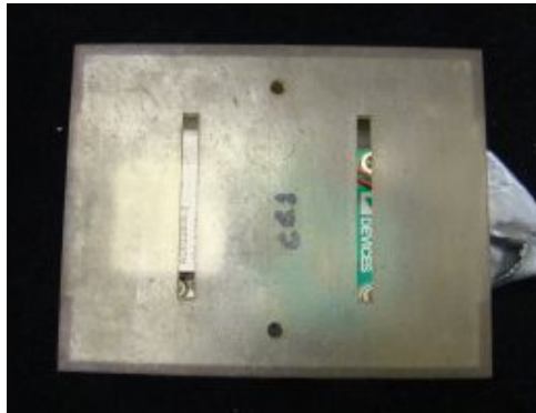
Figure 11: ADIS16250 Torso Mounting Box
