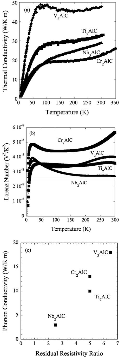
FIG. 5. (a) Temperature dependence of the thermal conductivity,  $\kappa$ . (b) Temperature dependence of Lorenz number. Note that the line near  $2.5 \times 10^{-8} \text{ V}^2/\text{K}^2$  is theoretical value for thermal conduction by charge carriers only. (c) Phonon conductivity,  $\kappa_{\text{ph}} = (\kappa - L_0 T / \rho)$  versus residual resistivity ratio, indicating that  $\kappa_{\text{ph}}$  is dominated by scattering.
