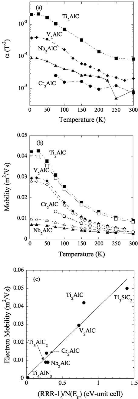
FIG. 3. (a) Semilogarithmic plot of  $\alpha$  as a function of temperature for several  $M_2AlC$  materials. The parameter  $\alpha$  was extracted assuming  $\Delta\rho/\rho(B=0) = \alpha B^2$ . (b) Temperature dependence of electron (solid symbols) and hole (open symbols) mobilities. (c) Mobilities at 4 K versus  $(RRR-1)/N(E_F)$ . The linear relationship indicates the electron-phonon coupling is similar in all studied  $MAX$  phases.
