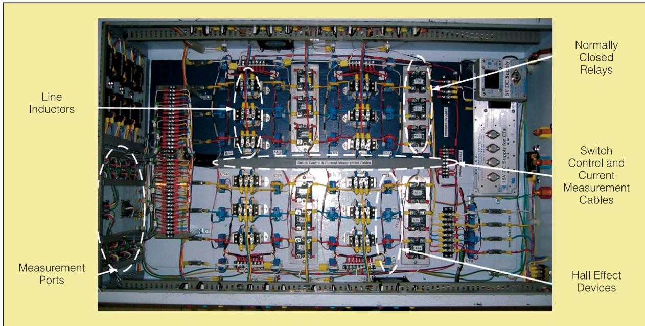
**Fig. 2.** Top-view of the Reconfigurable Distribution Automation and Control (RDAC) 9-bus distribution feeder box, showing power hardware and measurement hardware.
