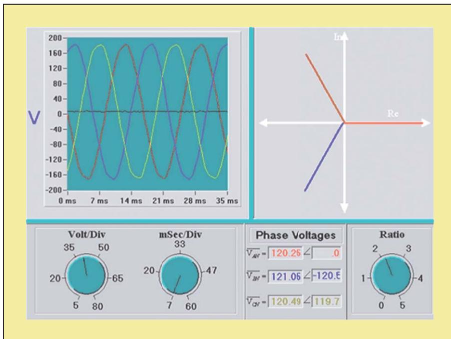
Fig. 8. Measurement instrument: oscilloscope view and the phasor diagram of three-phase ac voltages.
