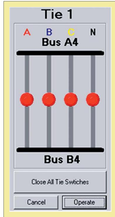
Fig. 9. Control instrument: network tie switch operation.
