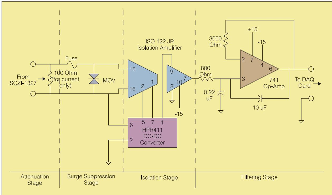
Fig. 4. Voltage and current signal conditioning circuits [9].
