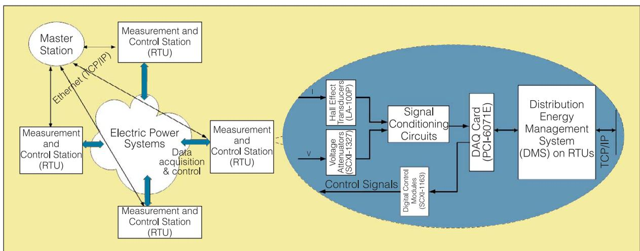
Fig. 1. System architecture of the measurement and control system.
