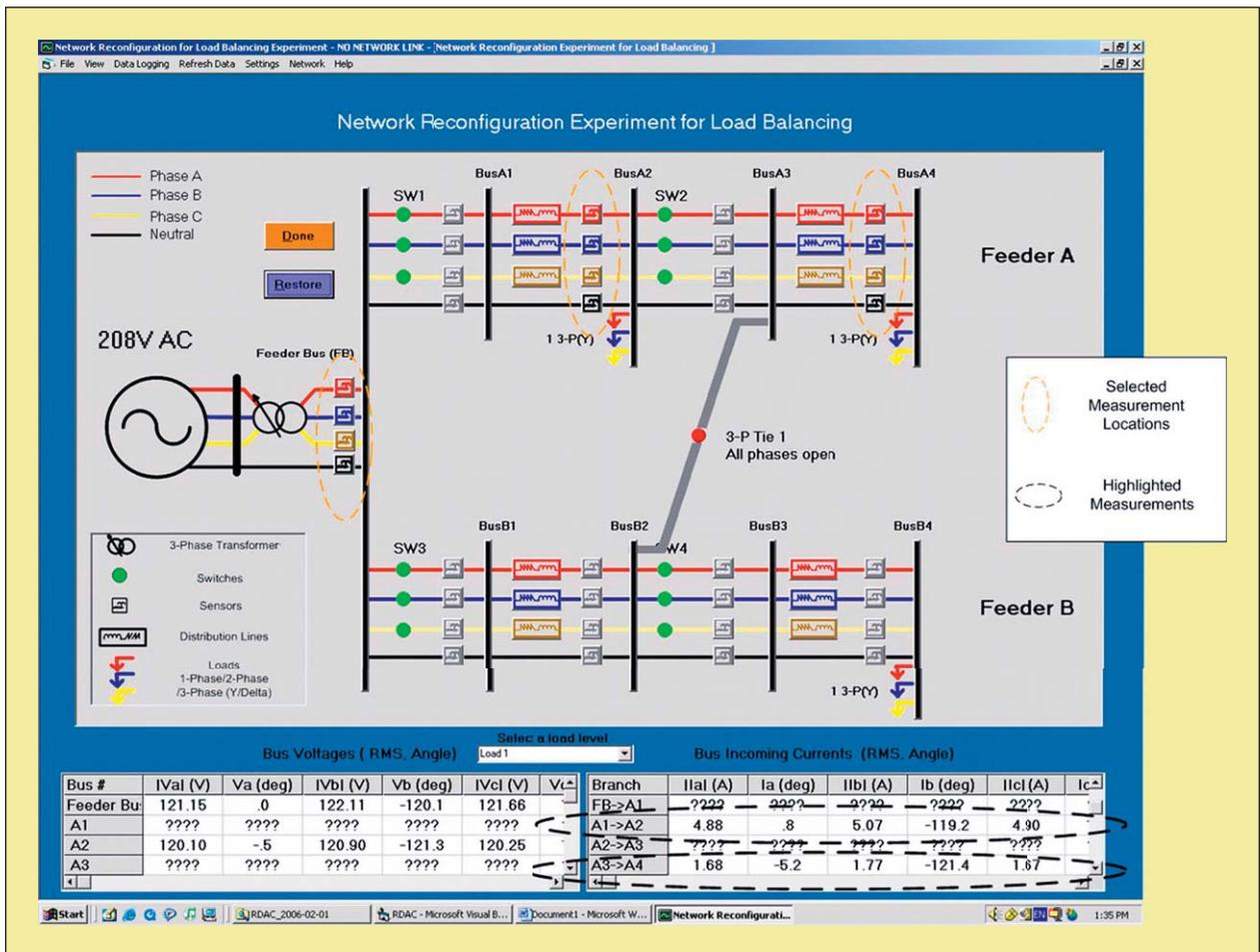
Fig. 11. A screen shot of the DEMS with selected measurement locations highlighted for load estimation.
