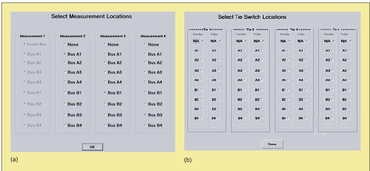
Fig. 6. (a) Measurement selection window with feeder Bus, Bus A1, Bus B1, and Bus B3 selected. (b) The tie switch location selection window.
