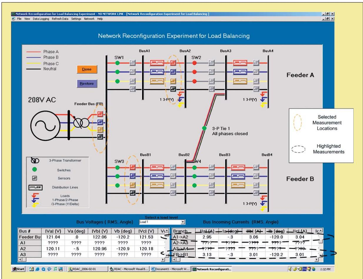
Fig. 10. A screen shot of the DEMS after network reconfiguration with SW2 open and 3-P Tie 1 closed.
