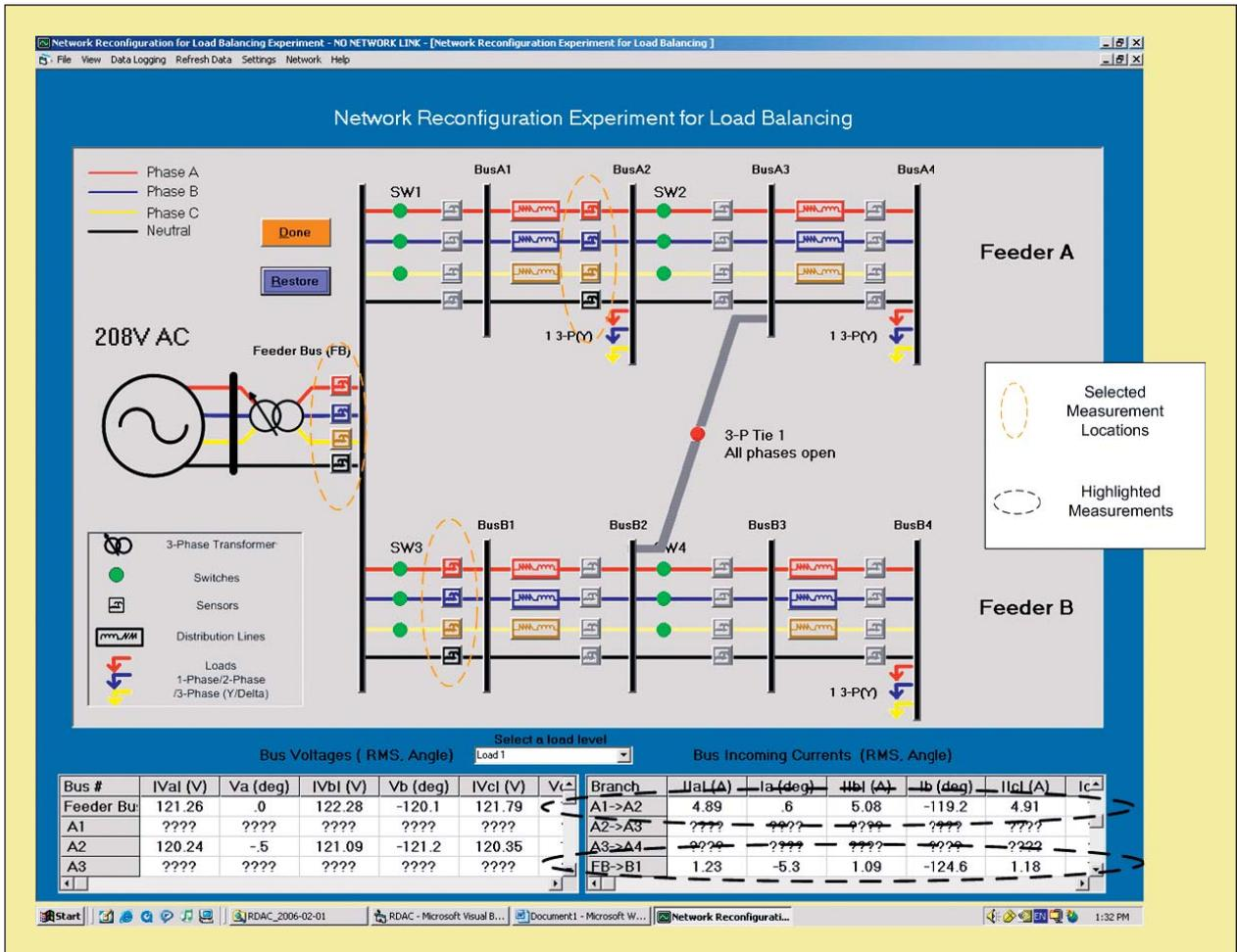
Fig. 7. Screen shot of the DEMS with selected measurement locations highlighted, before network reconfiguration.
