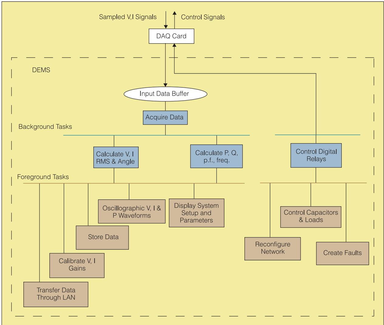
Fig. 5. The functional schematic of the Distribution Energy Management System.
