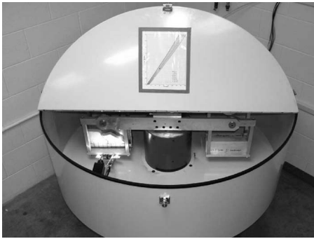
Fig. 1. Instructional centrifuge at Univ. of Colorado, Boulder. Photograph shows failed slope stability model in container to left (Photograph courtesy of Professor Dobroslav Znidarcic, used with permission).
