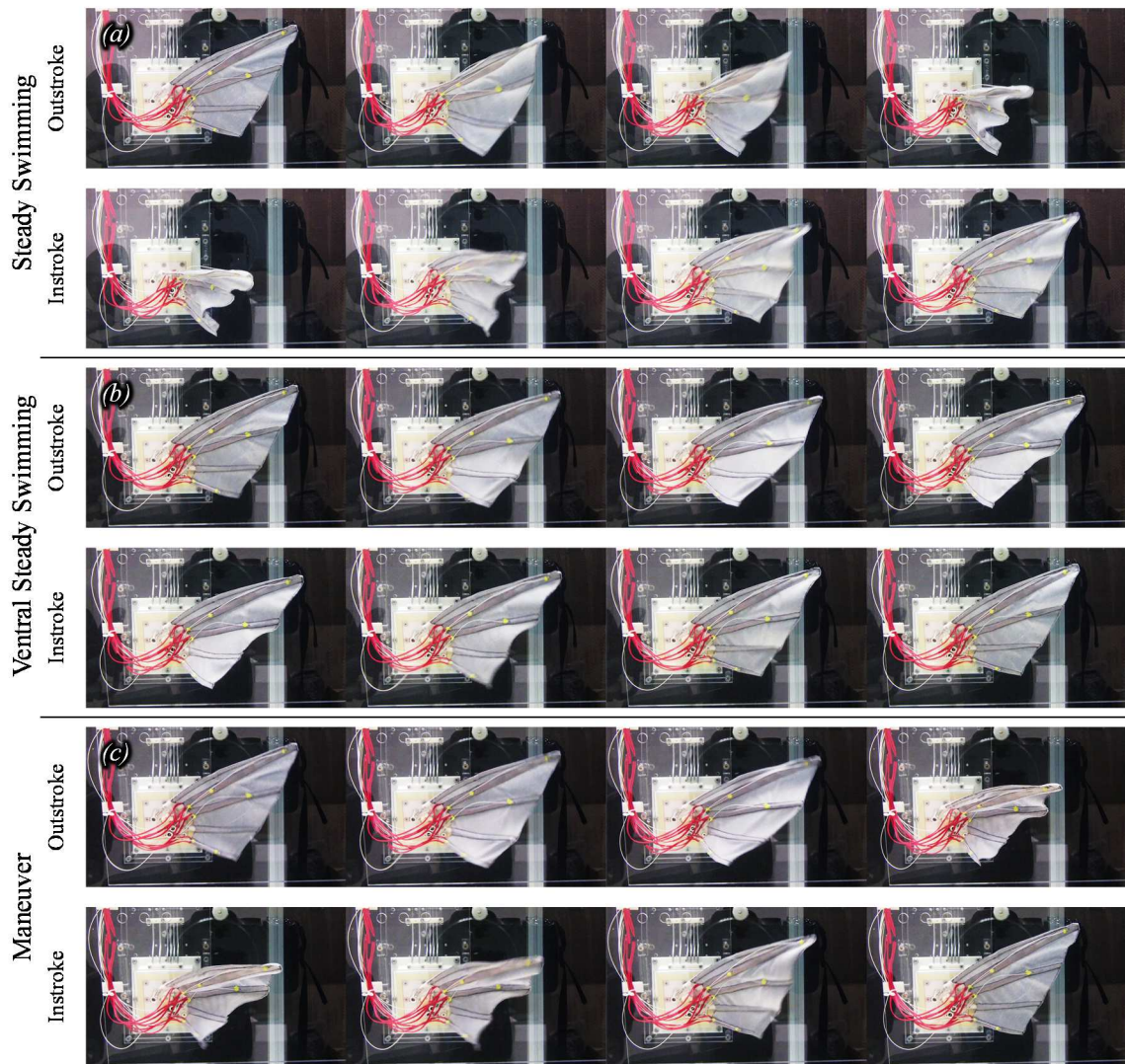
Figure 37. Picture summary of all gaits and stroke phases executed by the biorobotic pectoral fin in experiments. Gaits of steady swimming (SS; a), ventral steady swimming (VSS; b), and maneuver (M; c) were divided into outstroke (OUT, abduction) and instroke (IN, adduction) phases. Subsequent pictures were captured at time intervals of T/8 , where T was the sum of the outstroke and instroke execution times.
