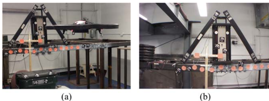
Figure 100. (a) UAS hovering near the steel deck. (b) Picture captured by the UAS camera
