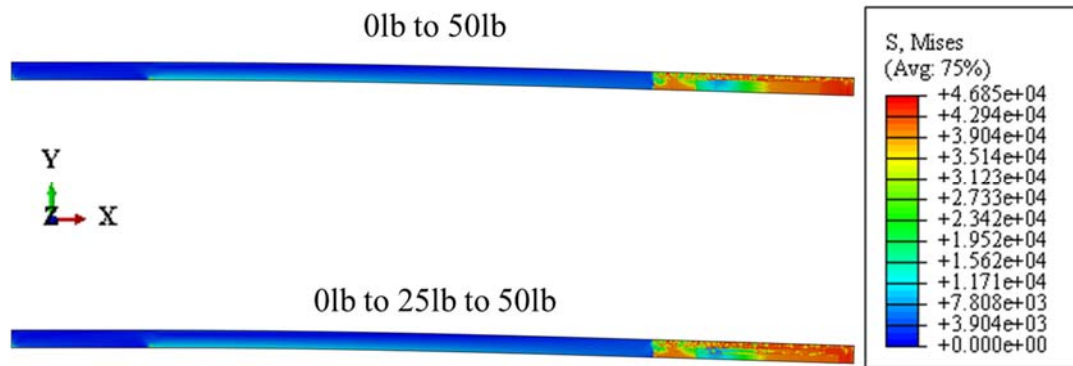
Figure 136. Stress comparison for different load paths from 0lb to 50lb (top) and 0lb to 25lb to 50lb (bottom)
