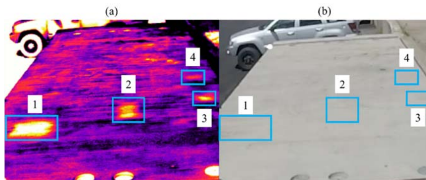
Figure 75. (a) Infrared image of the entire deck obtained with FLIR a325sc camera. (b) Color image of the entire deck.
