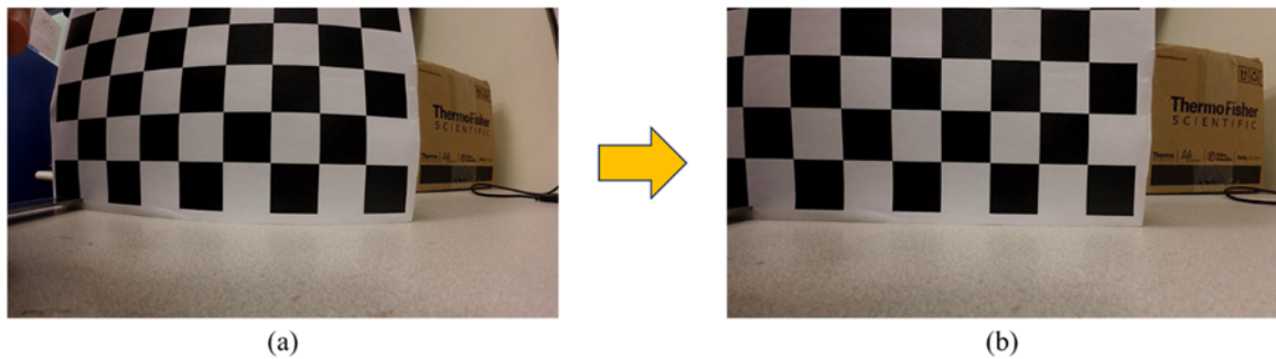
Figure 48. Results of GoPro lens distortion correction
