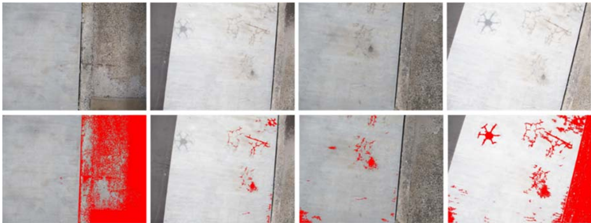
Figure 82. Color images captured during flight (top row) and post-processed images (bottom row)
