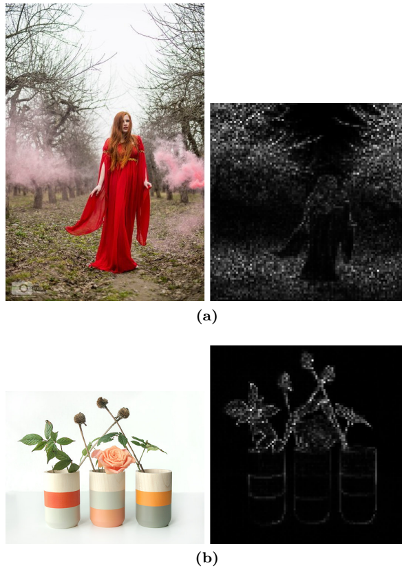
Figure 3.5: The Laplacian image for computing spacial edge distribution for two images. The feature for figure a. is 0.013 and for b. is 0.30.
