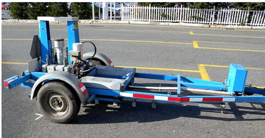
Figure 5-11: Original FWD Trailer Purchased in June, 2011
