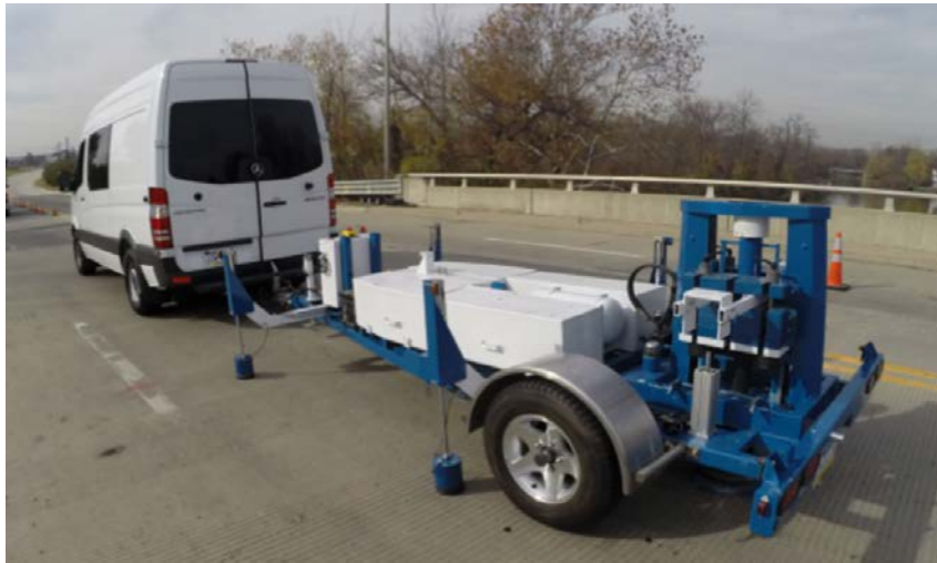
Figure 10-2: The Targeted Hits for Modal Parameter Estimation and Rating (THMPER) System
