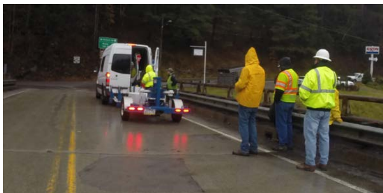
Figure 7-23: THMPER System Test on Mossy Interchange Bridge
