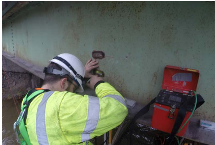
Figure 2-1: Strain Gauge Installation
