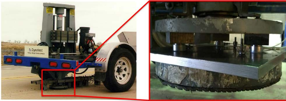
Figure 5-13: Falling Weight Deflectometer Load Cell Installation
