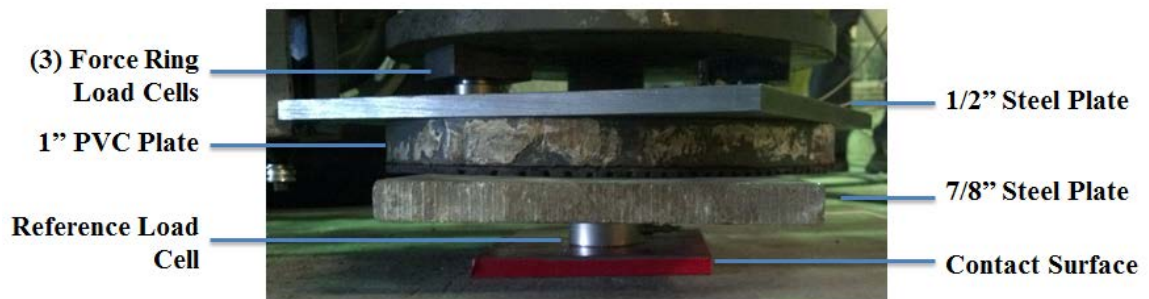
Figure 5-15: Load Cell Assembly – Benchmark Test
