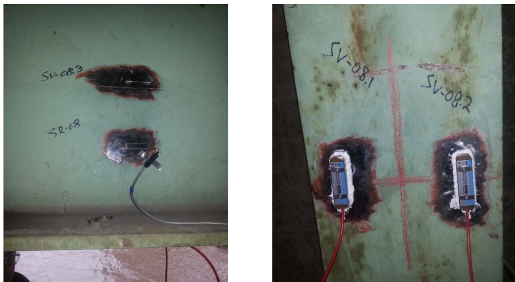
Figure 7-51: Strain Gauge Web Installation – Web
