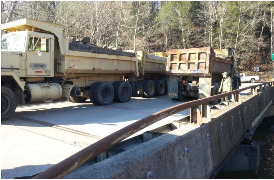
Figure 7-52: Positioning Trucks during Proof Loading
