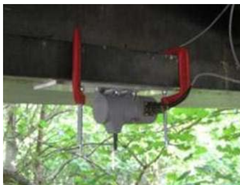
Figure 7-49: Typical String Pot Installation
