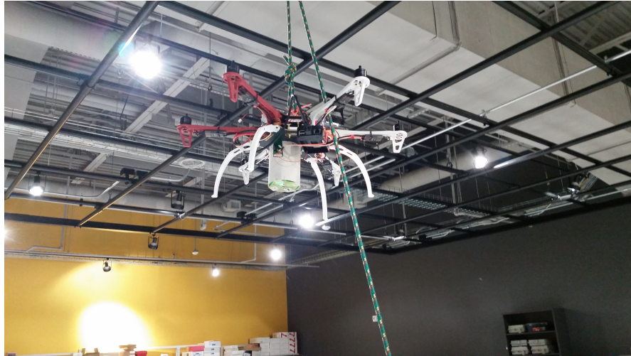
FIGURE 7.2: UAV hanging from ceiling grid during non-flight scenario experiment
