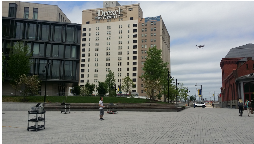
FIGURE 10.4: Experimental flight with reactive jammer (leftmost cart), ground node (rightmost cart) and UAV in the air on the right-hand side of the image
