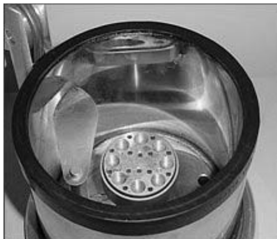
Figure 2.6 Denton II sputter coater.
