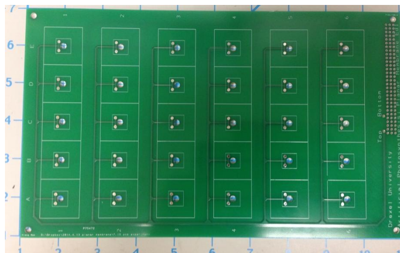
Figure 3-50. Photo of PCB fluidic testing board for ion channels on planar membrane.
