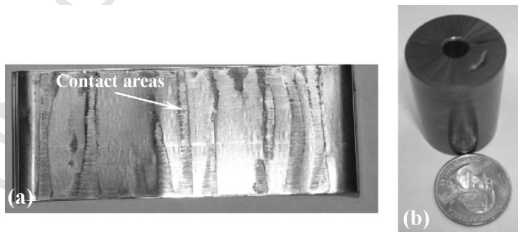
Fig. 11. Pictures of: (a) Ni-based SA top foil, and, (b) TaAgR shaft after testing in the air-foil bearing rig.
