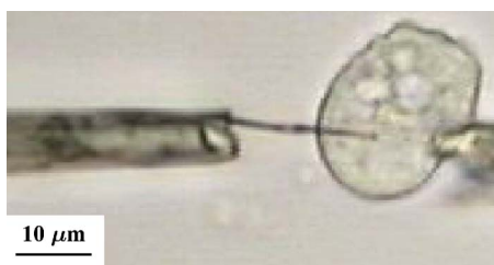
FIG. 4. Optical image of a nanotube tipped pipette (left) is injected into a MDCK cell held in place by negative pressure on a patch pipette (right). Negligible deformation of the cell occurs.
