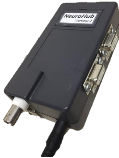
Figure 1 NeuroHub core module with 4 RS232 ports, 1 TTL port, and 1 parallel port
