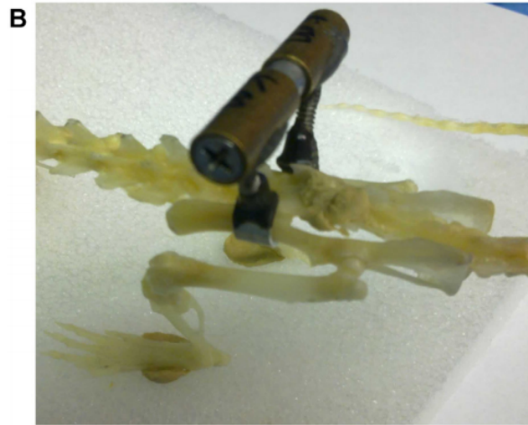
Figure 2-1. Custom-made pelvic orthosis placed on the pelvis of a rat skeleton, demonstrating how it interacts with the animal. Used with permission from Udoekwere et al., 2014
